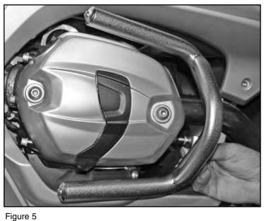
**4.** Loosely install engine guard at lower mount hole using one each:
