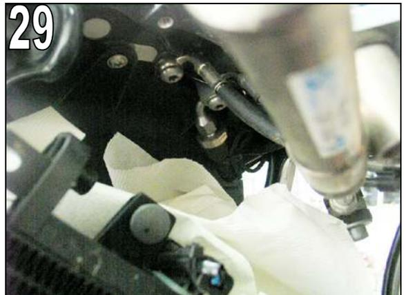
First detach control unit connection, remove hollow bolt, fit new sealing rings and attach brake line supplied using the 75° connection. Neutralise any escaped brake fluid immediately.
