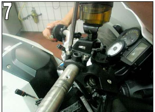
**WARNING: Air in the brake system leads to malfunctions. Support or suspend the brake fluid reservoir so that no air from the reservoir can enter the line system!!! Brake fluid can damage painted surfaces!!! Protect painted surfaces from damage using suitable means!!!**
