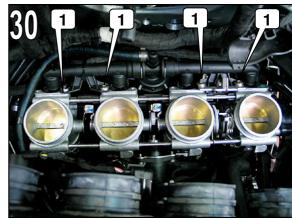
Unclip closing throttle cable (1), extract. Fig.31)
