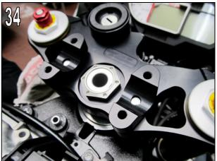
To tighten the lock nut, use a 12-sided socket. Depending on design, fit film tape to flange to prevent damage to the anodized coating (Fig.35).
